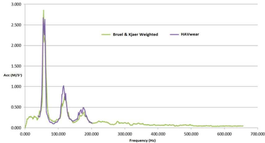
Fig 3 Correlation of frequency domain acceleration data from Bruel & Kjaer Photon + and Reactec HAVwear device
