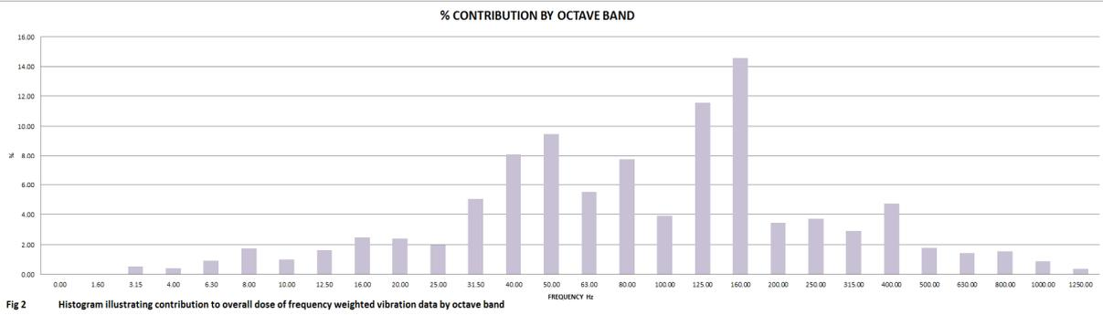
percentage of overall vibration magnitude across 27 commonly used vibrating tools of different action, mass operating speed and input power source. Vibration at frequencies greater than 650 Hz make up less than 3% of the overall weighted vibration, therefore the reduction in spectral range employed by the wearable device to conserve battery life does not have a material influence on the validity of data acquired.
