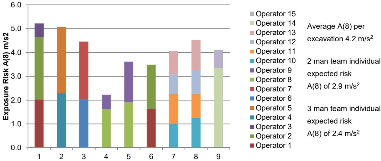
Figure 5 Calculated total exposure in A(8) m/s<sup>2</sup> for each excavation
