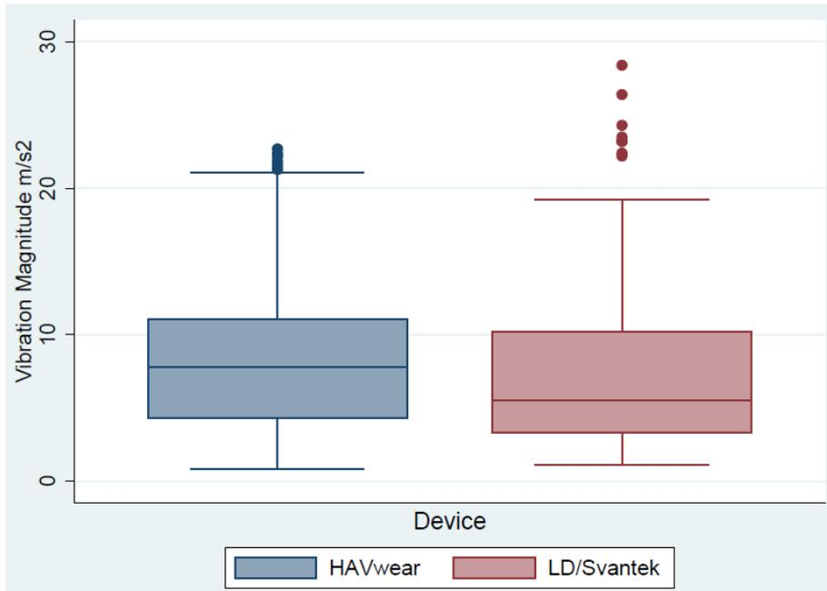
**Figure 3.4 – A boxplot comparison of the HAVwear and LD/Svantek without the results from the Makita HR2610.**
