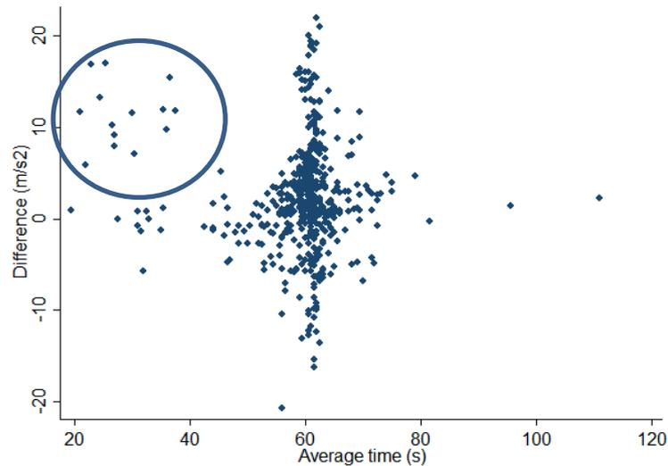
**Figure 4.3 - A comparison of the difference in vibration magnitudes for each test (HAVwear - LD) by average time recorded by the two devices. The encircled data is from the 1" impact wrench tests.**
