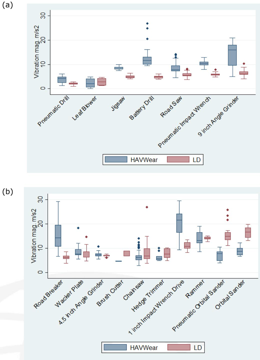
Figure 4.1 - The distribution of HAVwear and LD measurements for each tool where measurements are (a) lower and (b) higher than the overall LD median (6.24 m/s<sup>2</sup>).
