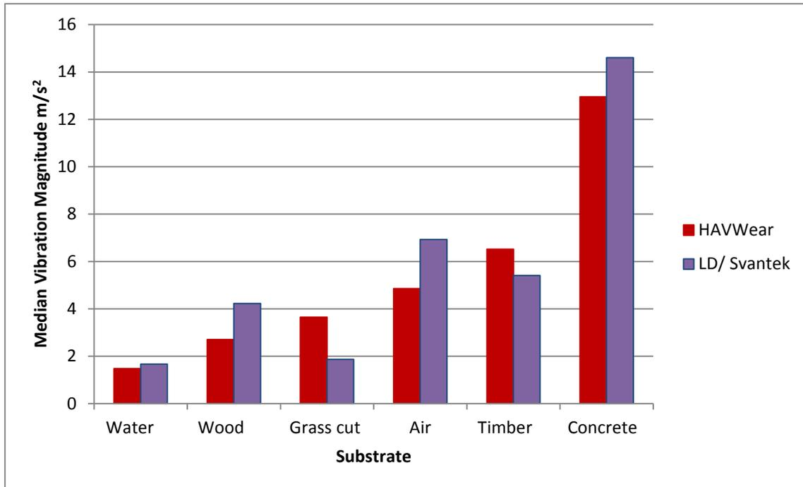
**Figure 3.6 – Vibration magnitude measurements in different substrates.**
