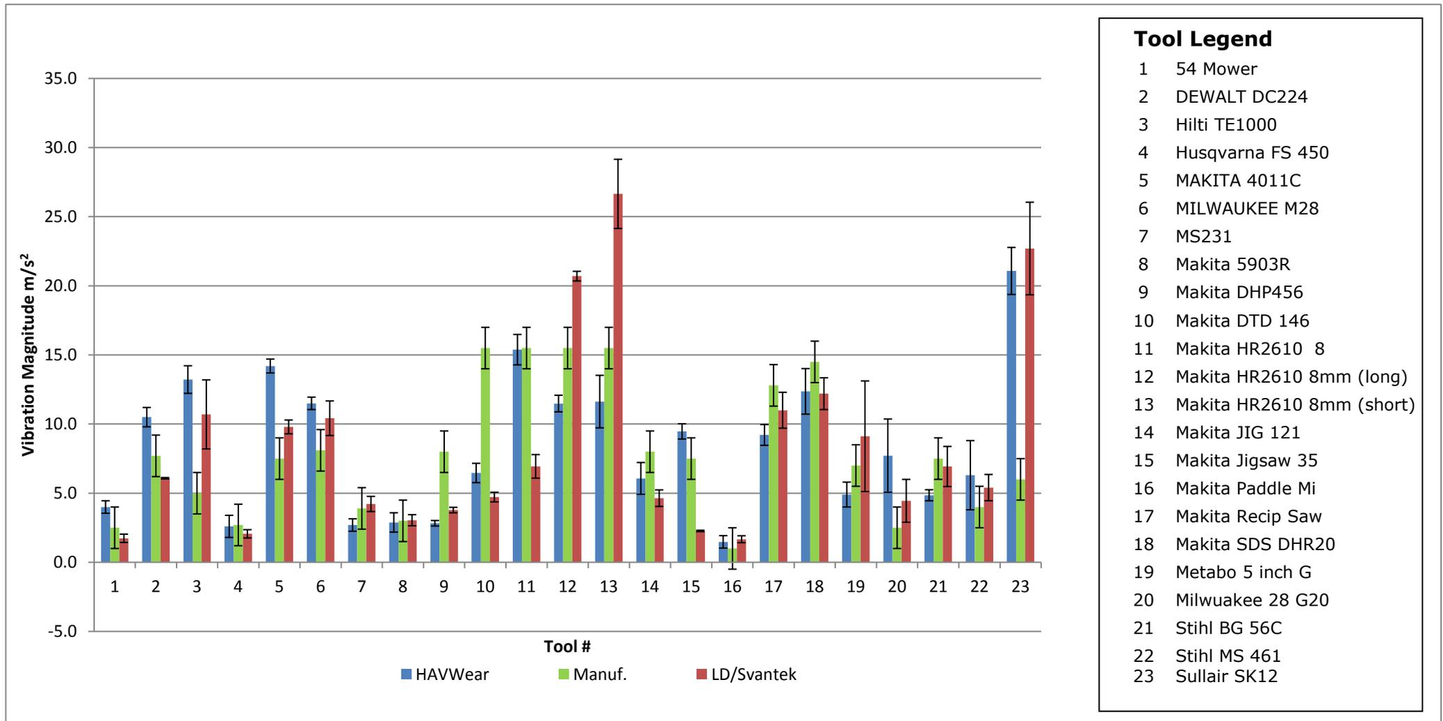
Figure 3.5 – The median vibration magnitudes measured by HAVwear and LD or Svantek alongside manufacturer values.
