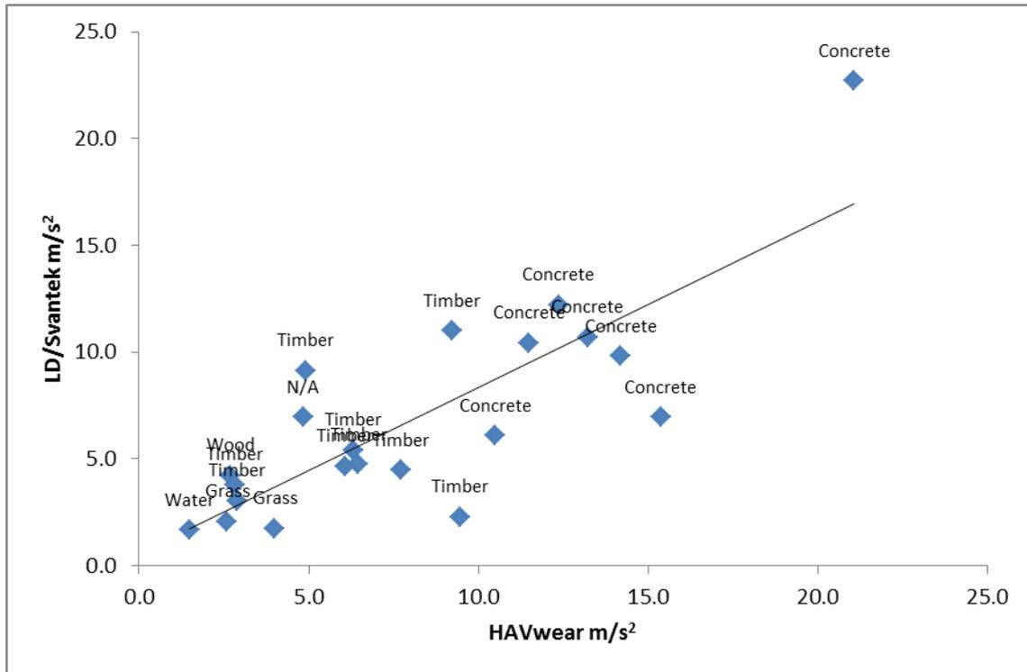
**Figure 3.2 - The correlation between median HAVwear and LD/SvanteK readings, with test substrate, omitting test tools #12 and #13.**
