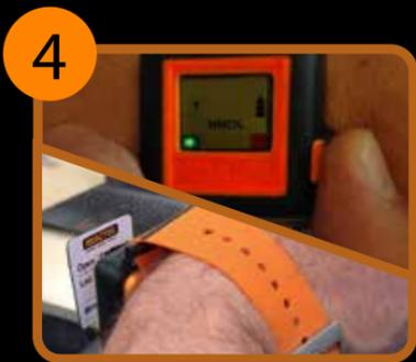
4. To "connect" to a SAFE-ZONE press the button on the HAVwear once, place the HAVwear over the SAFE-ZONE tag until a beep sounds. The display will show "SAFE" to indicate social distance detection is switched off
