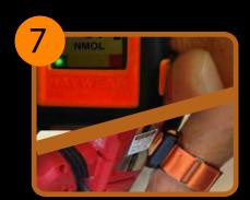
**7.** Before using each tool, press & release the HAVwear button once before placing the HAVwear over or on a tool tag until a beep sounds, to "Connect" to the tool. The display will show the first 4 characters of the tool ID to confirm connection.
