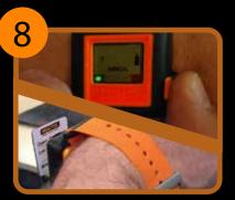
**8.** To "connect" to a SAFE-ZONE press the button on the HAVwear once, place the HAVwear over the SAFE-ZONE tag until a beep sounds. The display will show "SAFE" to indicate social distance detection is switched off
