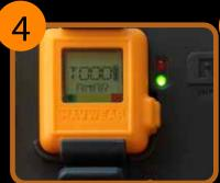
**4.** Remove the ID card and the HAVWEAR will display the first name initial and first three letters of the ID card owner's last name.
