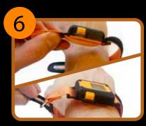
**6.** Insert the HAVwear into the holder so only the strap is in contact with the wrist. Snugly fit the strap around the wrist (do not remove until returning to a Docking station).
