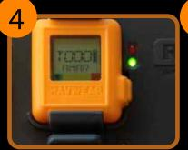
**4.** Remove the ID card and the HAVWEAR will display the first name initial and first three letters of the ID card owner's last name.
