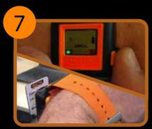
7. To "connect" to a SAFE-ZONE press the button on the HAVwear once, place the HAVwear over the SAFE-ZONE tag until a beep sounds. The display will show "SAFE" to indicate social distance detection is switched off
