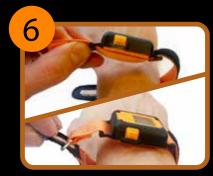
**6.** Insert the HAVwear into the holder so only the strap is in contact with the wrist. Snugly fit the strap around the wrist (do not remove until returning to a Docking station).
