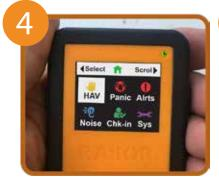
4. The main menu button controls are displayed at the top of the screen to navigate and select the menu options below.
