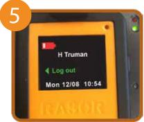
5. To return a RASOR, place the device onto a dual charger. Press the left button to log out. Do not log out if RASOR is to remain assigned to gather data. RASOR will auto log out 4 hours after being placed onto the Dual Charger.
