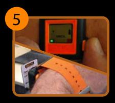
5. To "connect" to a SAFE-ZONE press the button on the HAVwear once, place the HAVwear over the SAFE-ZONE tag until a beep sounds. The display will show "SAFE" to indicate social distance detection is switched off.
