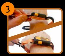
**3.** Insert HAVwear into the holder so that the strap is in contact with the wrist. Snugly fit the strap around the wrist (do not remove until returning to a Docking station).
