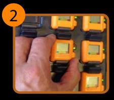
**2.** Unclip the HAVwear from the bay with the flashing LED light.
