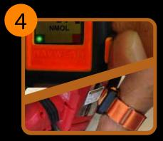
**4.** Before using each tool, press & release the HAVwear button once and place the HAVwear over a tool tag until a beep sounds, to "Connect" to the tool. The display will show the last 4 characters of the tool ID to confirm connection.
