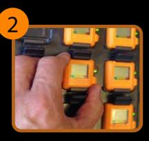
**2.** Unclip the HAVwear from the bay with the flashing LED light
